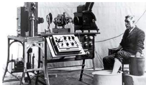
Figure 1 – Willem Einthoven making use of the novel electrocardiograph devised by himself in 1903
