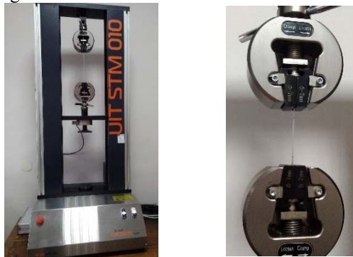
Fig. 6. Laboratory testing of tissues and biomaterials using Smart Tensor UIT STM 010 and sample from a rubber-plastic tube
