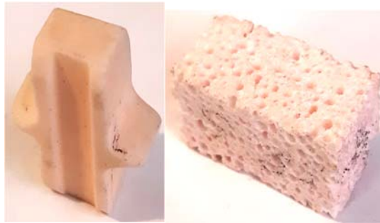
Fig.3. The appearance of \text{Al}_2\text{O}_3 : (a) monolithic and (b) porous
