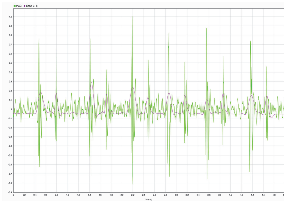
Fig. 14. The red line (emd_3_8) represents the smooth signal obtained after the addition of 3 to 8 IMFs of the EMD corresponding to the envelopgram. The green line is the original PCG.
