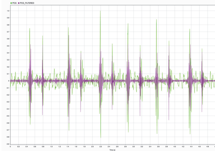
Fig. 12. PCG signals before (green line) and after (purple line) the band-pass filter.
