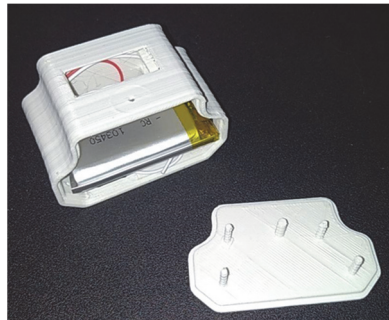
Fig. 18. Physical prototype of body and cover.
