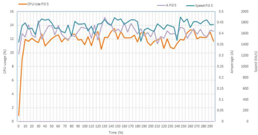
Figure 6: Comparison of CPU usage, power consumption, and file download speed of RPi 3
