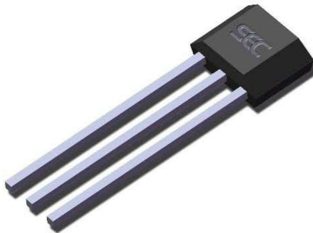
Figure 4: Hall sensor SS41F from SEC Electronic Inc. in 3-lead SIP package [13]
