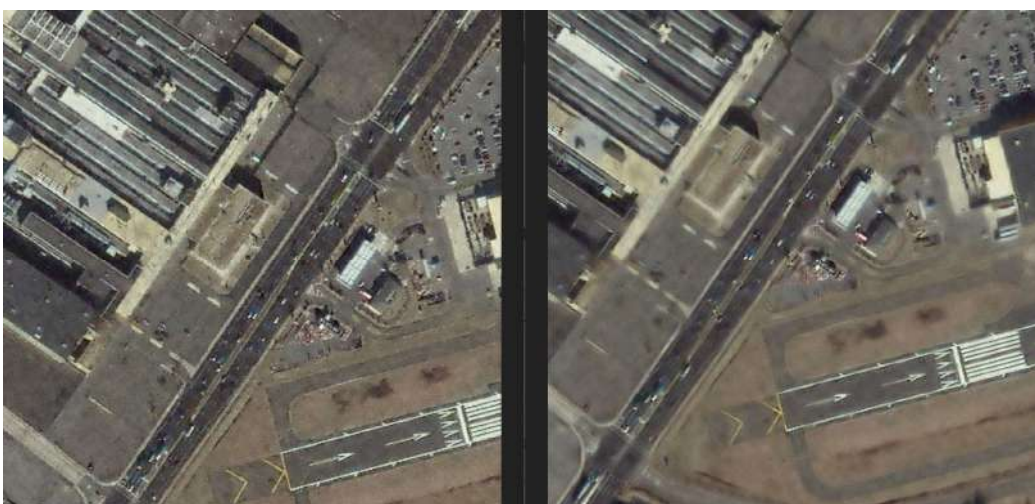
Figure 4: Comparison of 6 fragments of the image after noise reduction using KNN (left) and NLM (right)
