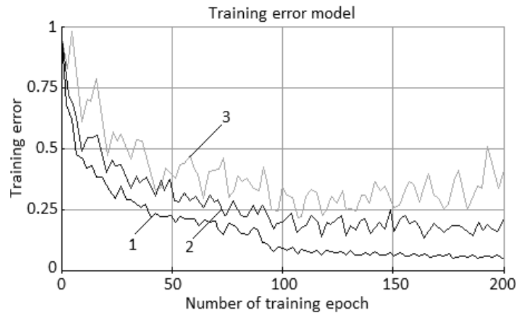
Figure 3: Comparison of the percentage of errors of classical neural network architectures designed for control complex dynamic objects: 1 – recurrent neural network; 2 – multilayer perceptron; 3 – convolutional neural network
