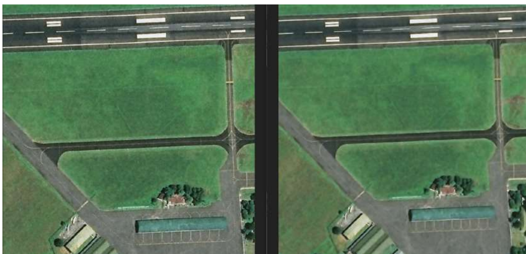
Figure 5: Comparison of 8 fragments of the image after noise reduction using KNN (left) and NLM (right)
