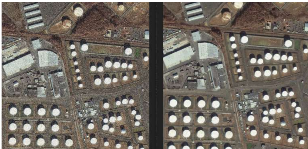
Figure 2: Comparison of 5 fragments of the image before (left) and after (right) noise reduction using the KNN algorithm
