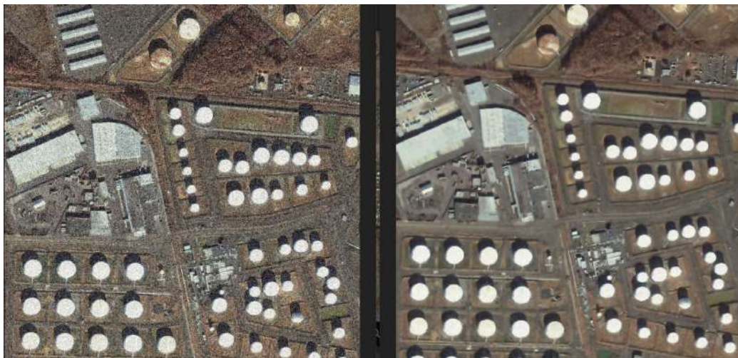
Figure 3: Comparison of 5 fragments of the image before (left) and after (right) noise reduction using the NLM algorithm
