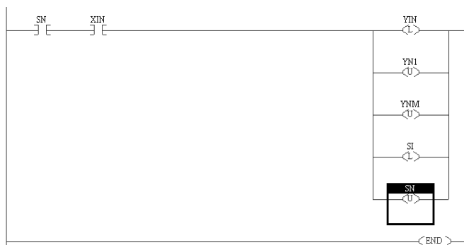
Figure 6.7. – Programming of the Mealy machine according to the principle of “all ingoing” a – a fragment of the graph with ingoing arcs incident to the state of S_i ; b – part of the program
