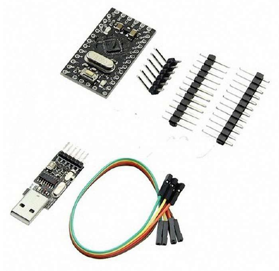
Fig. 5. Set of the Arduino board, converter and some connectors
