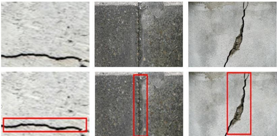
Figure 4.17 - Examples of concrete crack detection based on low-power embedded equipment
