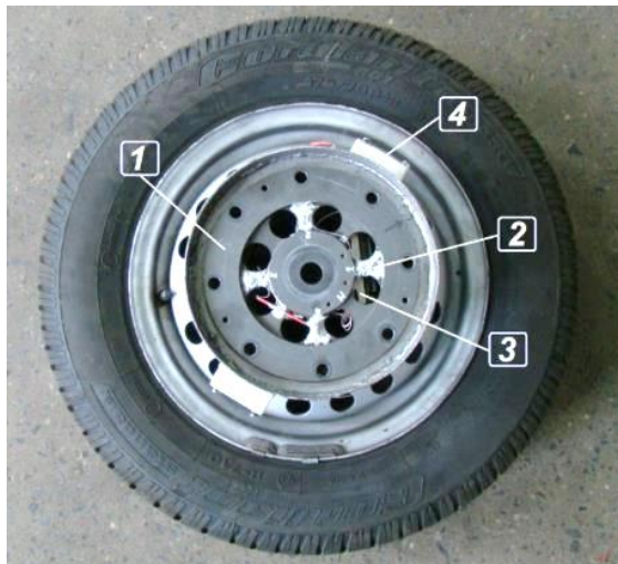
Figure 3. Equipment for measuring side force on the steered wheels, 1- measuring ring; 2- strain gauge with a protective layer of sealant; 3- adjustment board; 4- power supply
