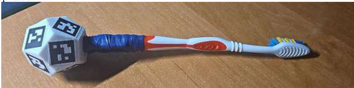
Figure 3: Our proposed modified toothbrush for 6DOF tracking
