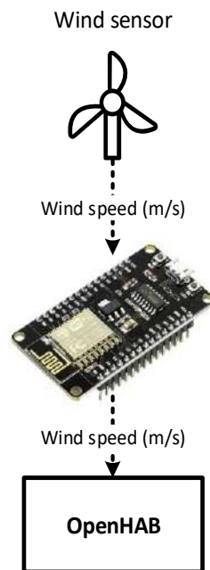
Figure 4: Architecture of custom wind measurement system
