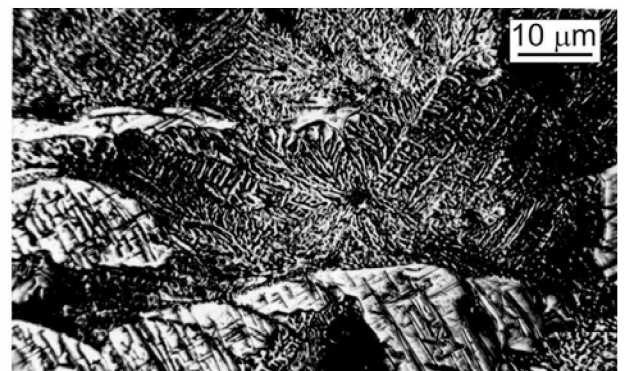
Fig. 4. Nucleation and growth the second eutectic \gamma\text{-Fe} phase (austenite) on the terrace of primary \text{Fe}_3\text{C} crystal
