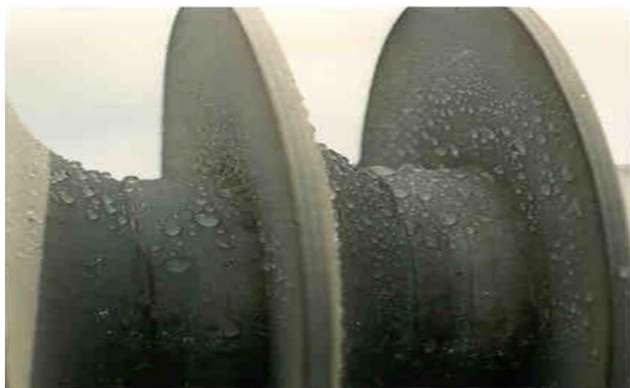
Figure 3.6 – High Hydrophobicity of the polymer insulator
