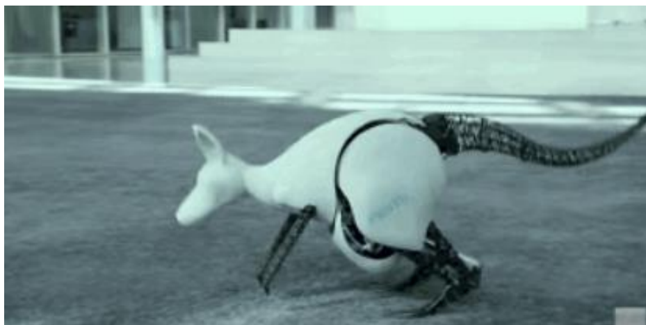
Figure 5.4 – Bionic Kangaroo Robot
