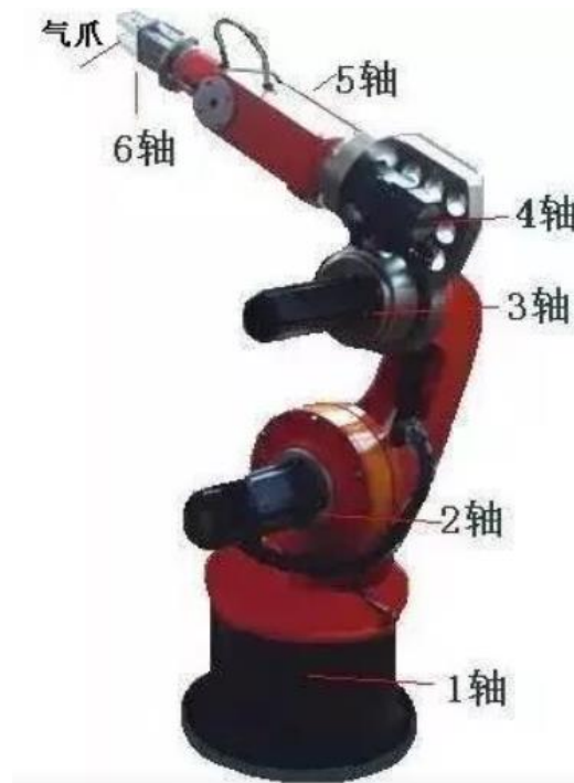
Figure 5.5 – Joints of a six-axis industrial robot
