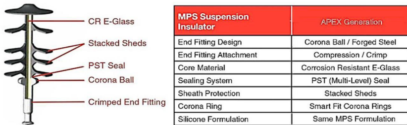
Figure 2 – Design of MPS Insulator [4]
