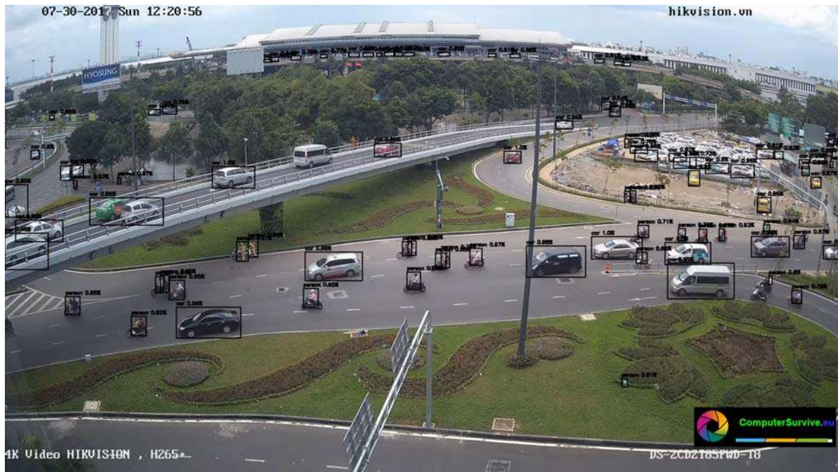
Figure 4: Examples of object detection on a 4K image based on proposed algorithm
