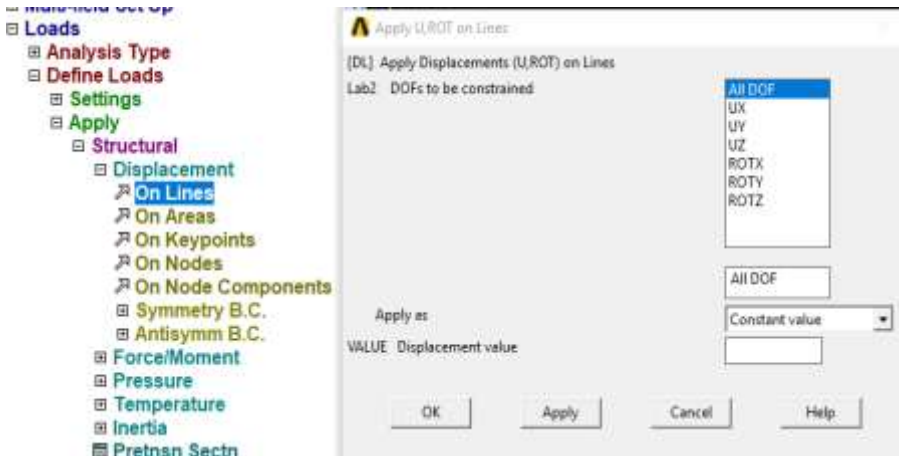
Figure 5.9 – Application of boundary conditions
