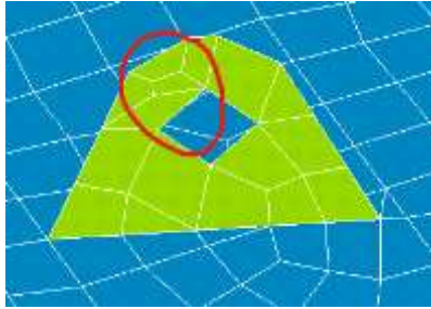
Figure 7.4 – An example of an irregularly shaped element that can lead to a calculation error
