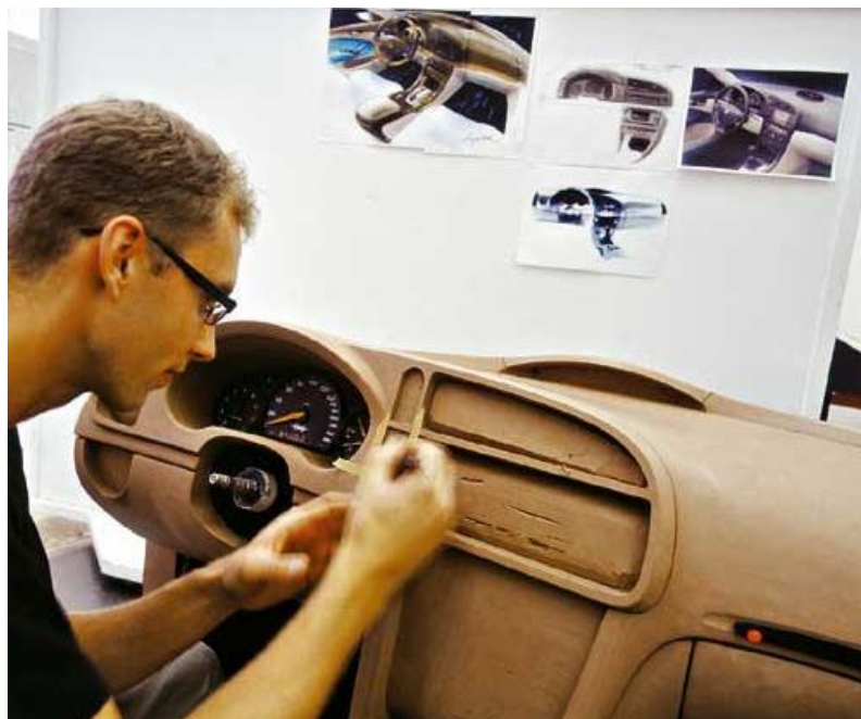
Fig. 6.5. Designing a dashboard layout
