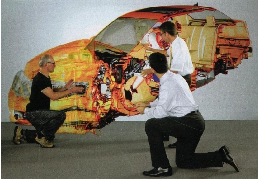
Fig. 14.9 Analysis of the results of a «virtual» car crash test
