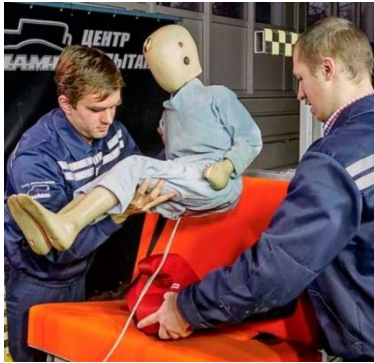
Fig. 7.13. Positioning the child dummy on the seat
