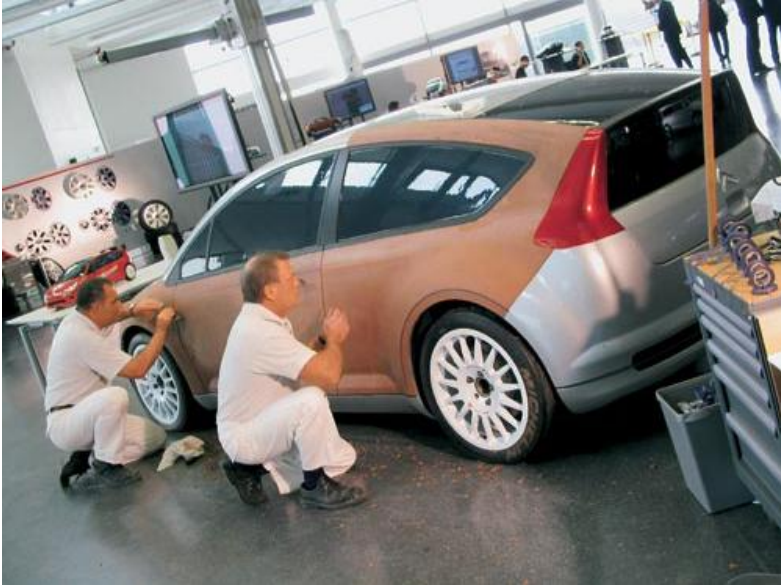
Fig. 6.4. Work on the car body mock-up
