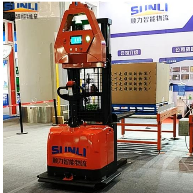
Figure 1.4 – Unmanned Handling Forklift Automated Guidance Vehicle
