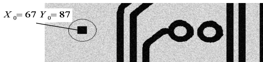
Fig. 7. Fragment of the PCB image and the result of localization of reference marks
