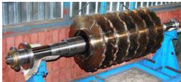
Fig. 1. A rotor of the multistage centrifugal compressor 225GC2-135/12-50M1245.
