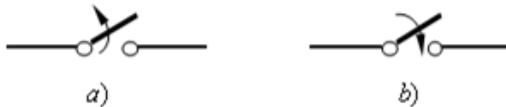
Fig. 6.1, a - a switch is to be opened, and b - a switch is to be closed.
