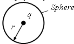
Fig. 1.6. Configuration for deriving Gauss's electric flux law
