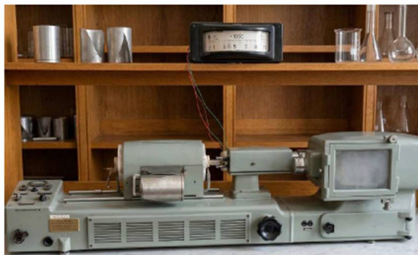
Fig. 1 – Photo of the Chevenard dilatometer setup
