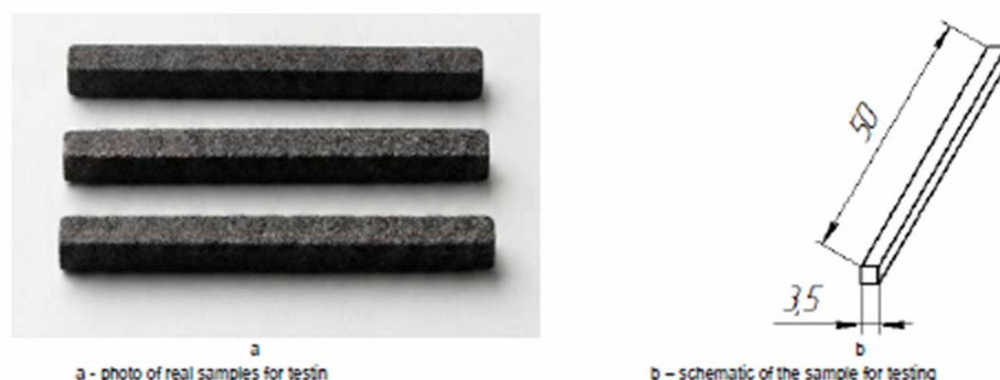
Fig. 2 – Samples for investigating the coefficient of linear thermal expansion
