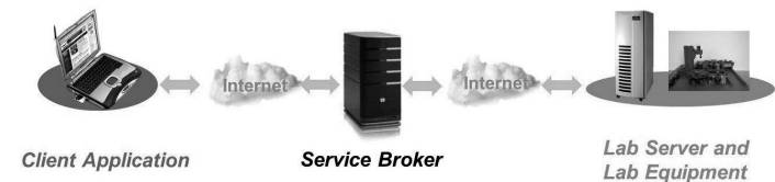
Figure 3. iLab Shared Architecture of the MIT (4)
