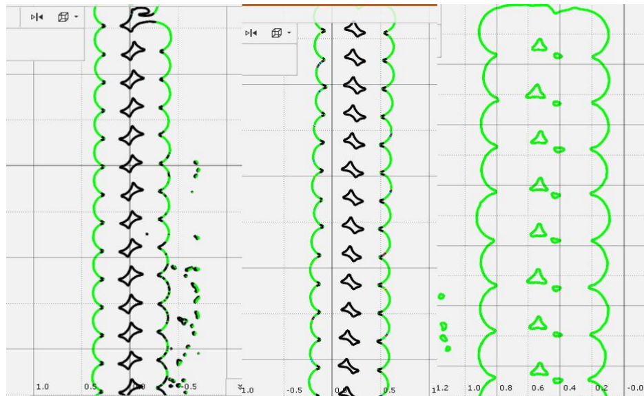
Figure 3.24- The geometry of top layers' cross-sections with: a) no NBD shift; b) +0.8 shift; c)-0.3 shift
