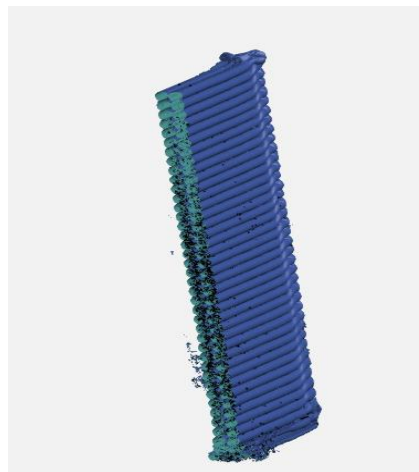
Figure 3.22- The cross-section of the specimen with no NBD shift in GOM Inspect
