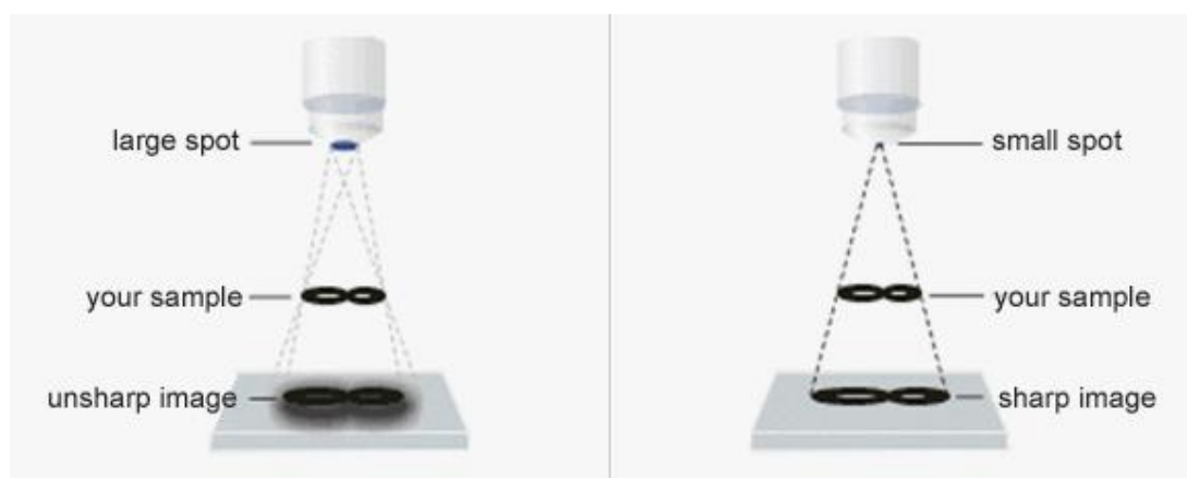
Figure 3.8-The influence of focal spot size on the CT scan accuracy
