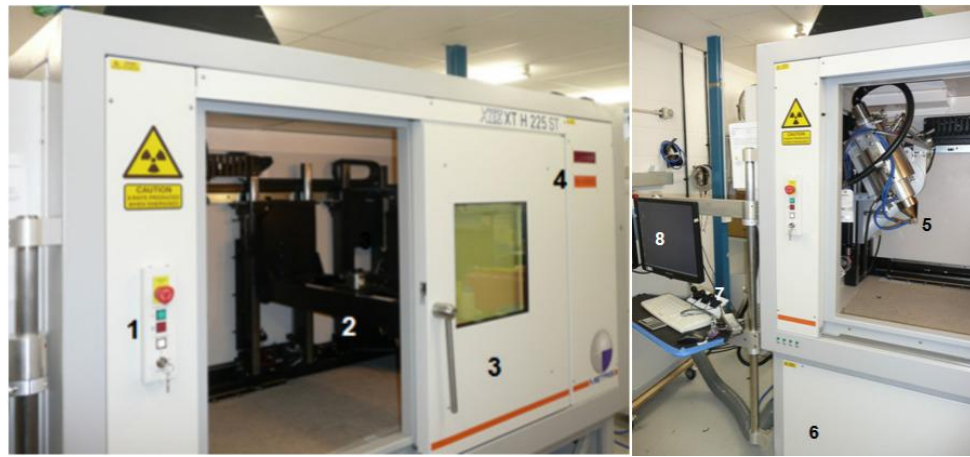
Figure 2.4 - CT system Nikon XT H225ST: 1) stop panel; 2) manipulator; 3) sample-loading door; 4) “X-ray ON” Lamp; 5) X-ray source; 6) service access panel; 7) manual joystick controls; 8) LCD monitors
