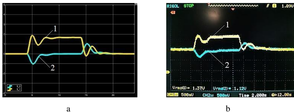
Figure 5. Graphs of the transients of the position of the first \varphi_1 and second \varphi_2 masses with the motor running and when applying M_r : a - mathematical model, b - physical model.
