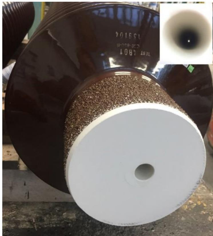
Figure 3.4– Support insulator with fiber optic hole after firing and cutting [44]
