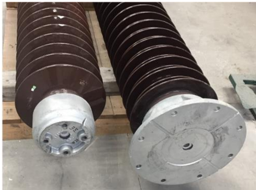
Figure 3.5 – Assembled C30-850 fiber optic support insulator ready for testing
